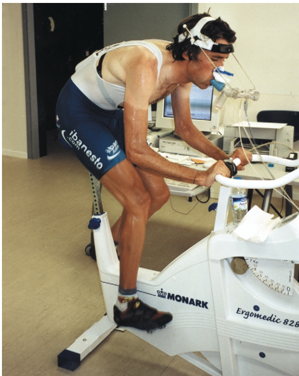
Figure 3. Measurement of maximum oxygen uptake in a trained cyclist during a cycle-ergometer test. The person breathes through a low-resistance mouthpiece, and the collected air passes through cables to a metabolic cart. The maximum oxygen uptake is an excellent indicator of functional capacity. Cancer patients have very low values, 48 about five times lower than those of trained athletes.
